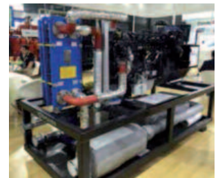
Gas Generator Set
